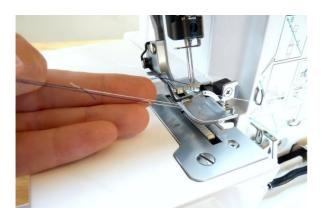
Keep pulling until the knots have strung through the whole machine and the new thread color has replaced the old.
