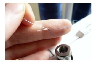
Tie the old color to the new color. I made a simple square knot and clipped the excess.
