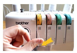
Pulling this knot through your tension discs is NOT a good idea. What I did is lower my tension down to zero then gently pull the thread up out of the discs. Pull the string of thread forward so the knot is now beyond the tension discs, then thread the new color back into the discs. Do this for all four.
