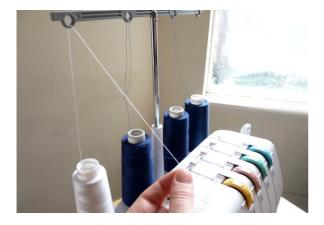
Replace your old thread with the new cones, and bring the new color through the thread guide.
