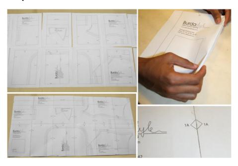
The patterns are printed out in letter sized pages within a thin frame. Wait until all sheets are printed out. Arrange the sheets so that they fit together (see additional page with the overview of the prints) following the markers. Fold the single sheets on the upper and right edge along the thin frame lines. Begin with the left lower sheet and then tape the frame lines together precisely.
