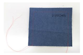
This photo shows the corner cut by 2 stitches on medium weight fabric.
