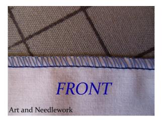
The serged sample I am using in the photos is a three-thread overlock stitch where medium blue thread was used for the loopers and a navy for the needle.
