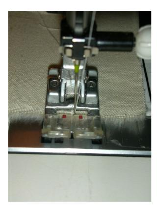
Sew to the very end of the strip. Leave the needle down and lift the presser foot.
