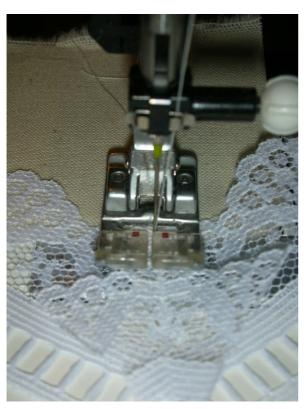
I'm zigzagging over the tiny seam in this lace. If I'd just put this in the sewing machine and prayed I'd get it out of there again nicely sewn, I would have been very disappointed. I butted the beginning of my difficult fabric at the end of my easy fabric, lowered the presser foot again, and continued to sew.
