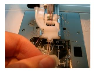
Bring the ends of the buttonhole twist under the foot and towards the front. Slide them in the guides at the front of your buttonhole foot. Again, this may vary by machine, so check your manual.
