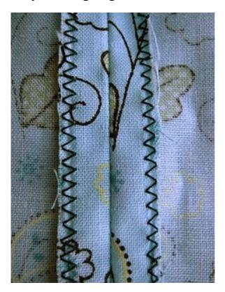
Sew a zig-zag stitch through the middle of each seam allowance. Trim each seam allowance as close to the zig-zag stitch as possible and press.
