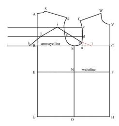
Measure the curved distance between point "b" and point "h" (i.e. the distance along the armhole curve), add 0,75 cm (5/16 in.), and swivel the straight-edged ruler around point "b" until it intersects the Armscye Line (the horizontal line passing through point "a") at this distance to the right of point "b". Mark this point "l" and draw in the line between "b" and "l".
