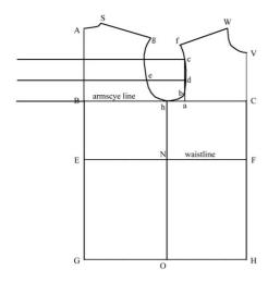
Where the horizontal line lift of point "d" intersects the back of the armscye line, mark the point "e". Also, let's change the designations for point Y to point "f", point U to point "g" and point M to point "h".
