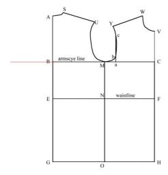
Now we are going to draw in three construction lines that will allow us to develop the sleeve cap (top of the sleeve). First we extend the Armscye Line to the left of point B.
