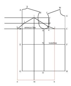
Now draw a horizontal line to the right of point "m" to the point "n" directly below point "l", and connect points "l" and "n". Then carry out a similar operation for the left size, drawing a horizontal line to the left of point "m" to the point "o" directly below point "k", and connect points "k" and "o".
