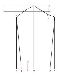
Halfway between points "m" and "q", mark the point "r". Now draw a short line 1 cm. (3/8 in.) straight down from point "r" and mark the point "s". Draw a vertical line straight up from the point "s" a full 10 cm. (4 in.) to point "t". This is where the sleeve slit will be located.
