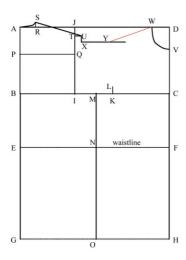
Measure the distance from point S to point U along the back shoulder seam and add 0,5 cm (3/16 in.). Pivot a ruler on point W so that it intersects with the horizontal construction line that runs through point X at this distance from point W, and mark this point Y. Draw in the front shoulder seam in a straight line from point W to point Y. The distance from point W to point Y is hence the distance from point S to point U plus 0,5 cm (3/16 in.).
