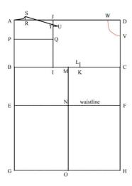
Measure one fifth the NECK size below point D and mark the point V. Measure one fifth the NECK size minus 1 cm (3/8 in.) to the left of point D and mark the point W. Draw in the neck curve boldly between points V and W.
