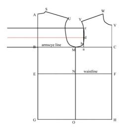
Halfway from point "a" to point "c", mark in an new point "d", and draw in another horizontal line left of point "d", the same length as the other two construction lines.
