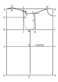
Connect points U, Q, M, L and Y with a curved line - this forms the armhole (also called the armscye). The curve should deviate a maximum amount of 1,25 cm (1/2 in.) outwards from the line connecting points L and Y at point Z, and should be inset roughly by 1,75 cm (11/16 in.) from point K on the diagonal inwards, and by 3 cm (1 & 3/8 in.) from point I on the diagonal inwards.
