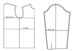
Like the sleeve block, the shirt block includes a 1 cm. (3/8 in.) seam allowance along the top edge only.
