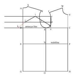
Measure the curved distance between point "e" and point "h" (i.e. the distance along the armhole curve) and add 1,25 cm (1/2 in.) - now swivel a straight-edged ruler around point "j" so that it intersects the Armscye Line (the horizontal line passing through point "a") at this distance to the left of point "j". Mark this point "k" and draw in the line between "j" and "k".
