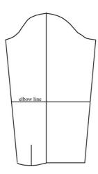
Now erase the various construction lines (or pencil in the sleeve outline in heavy pencil) to get the final sleeve block.
