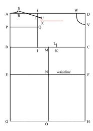
Draw a short construction line 2 cm (3/4 in.) vertically down from point U and mark the point X. Now draw a light construction line horizontally to the right of X about half way to the line CD.
