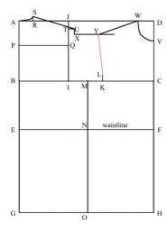
Connect points Y and L with a lightly drawn straight line. This is the construction line for the front part of the armscye (armhole).
