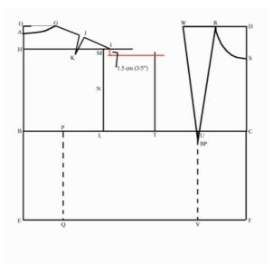
Shift your attention to the construction line passing through points H, M and I. Measure 1.5 cm (3/5") down and draw in lightly a new horizontal construction line across the middle part of the block.
