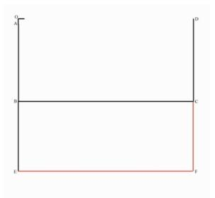
From point E, square across to and mark point F on the downward extension of the line CD. Note that the squaring may also be done by measuring the distance B to E and carrying this across to point C.
