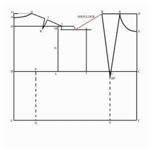
Now we repeat the pivoting measurement we did in Step 11 for the back shoulder. Using the SHOULDER measurement, fix the ruler zero at the point W and pivot the ruler until it crosses the construction line drawn in the previous step at the distance of the SHOULDER measurement, and mark this intersection (point X).
