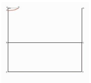
Draw a shallow upward curve from point A to point G - this is the back neck line. To draw the curve, if you don't own a French Curve (an extremely useful instrument for pattern making), you may use a dinner plate, but you will need to slide the plate along - draw a small segment, then slide the plate along and draw in the next segment, until you are able to reproduce the shape of the curve shown. This may take some practice on a separate piece of paper first.
