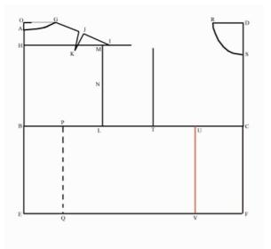
Find the halfway point (point U) between C and T and mark it (alternatively, the distance between C and U is half the bust separation - if this is very different than the norm, it will be important to include the appropriate measurement here). Then draw a dashed vertical line downwards to intersect line EF, and mark the intersection point (point V). This is the mid front line.
