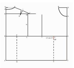
Mark the bust point (BP) at a distance of 2.5 cm (1") below point U. For some pattern manipulations, you will need to draw a horizontal line through the bust point from one side of the block to the other (the BUST LINE).
