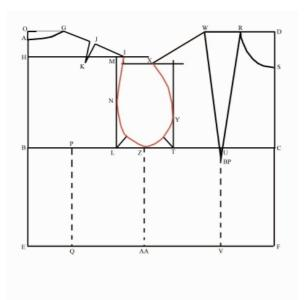
Using a French Curve or sliding dinner plate, draw in the ARMSCYE curve so that it passes smoothly through the construction points I-N-Lsegment-Z-Tsegment-Y-X. This completes the basic bodice block up to the construction of the waist line. If the garment is to be finished at the waist, then one should proceed to the final two steps in which the waist darts are constructed.
