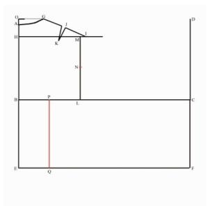
Find the point half way between L and M and mark it (point N). Also, find the point half way between B and L and mark this too (point P). Measure the distance from B to P and mark the same distance along the horizontal line from E (point Q). Draw a dashed line from P to Q.
