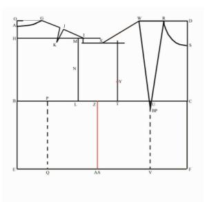
Measure upwards from point T, one third the ARMSCYE depth measurement and mark this location (point Y). Find the halfway point (point Z) between points L and T and mark this point. Draw a dashed vertical line down from this point until it intersects the waist line (line E to F), and mark the intersection (point AA).
