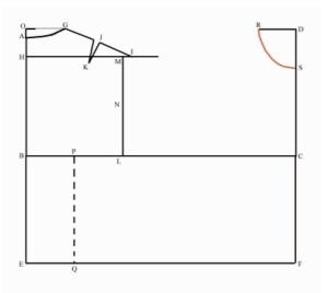
Draw a deep curved line from point R to point S, again, either using a French Curve or a sliding dinner plate. This is the neck edge on the front of the bodice.
