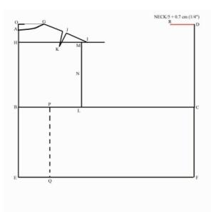
We now move from the construction of the back of the bodice block to the front of the bodice block. Starting from the point D, measure one fifth of the NECK measurement plus 0.7 cm (or 1/4") along the line connecting point D to point O and mark the resulting point (point R).
