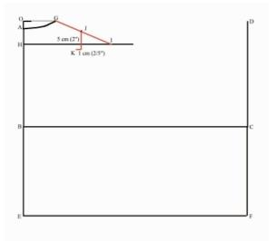
Next, find and mark the point half way from G to I along the shoulder (point J). From point J, measure 5 cm (or 2") down, and 1 cm (or 2/5") to the left. Mark this point (point K). This is the end of the shoulder dart.
