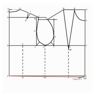
Extend the line from D to F downwards by from 0.5 to 1.5 cm, depending on the bust measurement (i.e. 1.5 cm for large bust sizes, 0.5 for small bust sizes and 1.0 for intermediate bust measurements) and mark the point (point AB). Draw a line from the point AB to the point E. This will be an oblique line. This extension ensures that the waist remains horizontal and doesn't ride up due to the bust.
