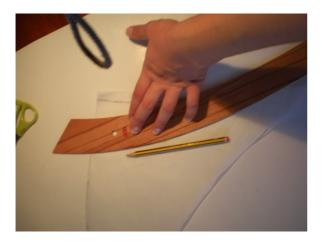
Put another piece of paper on the pattern and using the hp curve ruller, redraw the bottom line and all the other lines as they are.
