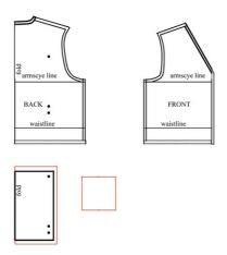
To complete the drafting of the pattern pieces, we add the seam allowances to the panel piece and introduce a rectangular piece of cloth for the battery holder. The size of this second piece is determined roughly by the size of the batteries we need to use. For the fiber optics cable I used, I
