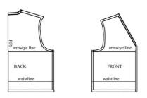
We have now arrived at the basic vest pattern. It should be noted that I lined the vest - this is a good idea, as we want to pack the electronics into the space between the lining and the outer material. So you will need to cut the vest pattern, front and back, out for both the outer fabric and the lining fabric. You might want to do this now, and sew the vest and lining together.
