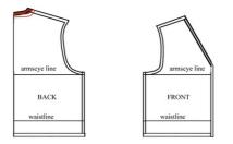
Because the front of the vest is left open, you will need to add a seam allowance to the center front line if you haven't already done so. You will also need to modify the back neckline slightly to conform to the changes made to the front neckline - essentially, broadening the "dipped" region so that the shoulder seam is the same length as found for the front block. Here, I've also added in the seam allowance.
