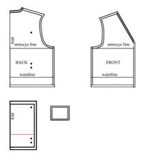
A final element to be drafted - I designed the back panel (see next step) to include a fabric "conduit" within which the fiber optics wiring is contained, running along the bottom of the panel. The seam line for this conduit is now shown in the diagram, slightly above the higher of the two snap fasteners located near the bottom of the panel.
