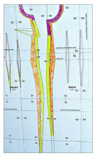
The ligt yellow markings demonstrate the zone beetween the new seam line and the line of the seam allowance. The light orange zone shows the volume of enlargement.
