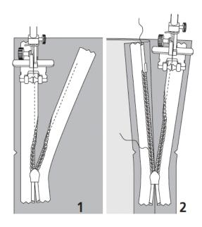
These special zippers come in various lengths. The zipper should be at least 2 cm (3/4 in) longer than the slit. It is sewn in place before the seam below the slit is stitched. A special presser foot is required to sew the zipper in place.
